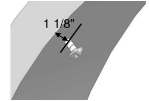
Insert the Bracket Clip into the screw from the notch.
