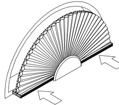
Place the front groove of the rail into the front iron wire of the bracket and then push forward to make the back groove of the rail snap into the back groove of the bracket.
