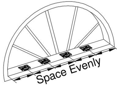
Use two #8x1 1/4" screws to attach the installation brackets on the window frame. The minimum distance is 11/16" from the front bracket to the edge of window frame.
