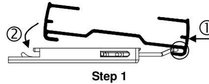
Insert the Bracket Clip into fabric and then close the Bracket Clip to keep it clamped on the fabric.
