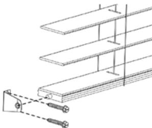
With the hold down brackets attached to the bottom rail, lower the blind to the hold down bracket mounting surface and mark the bracket locations.
