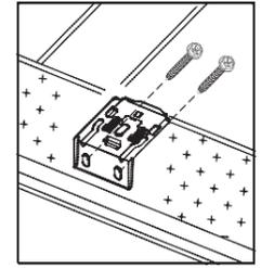
Make sure brackets are aligned. "L" shape opening should be facing down, with shorter side against the wall.
