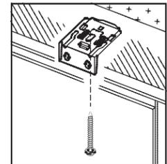
Make sure both brackets are aligned. "L" shape opening should be facing down, with longer side against top of the window opening.
