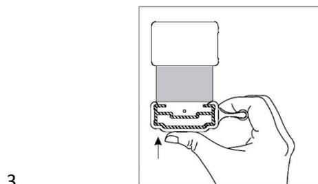
Transparent Cordless Handles should be operated from the center of the bottom rail.
