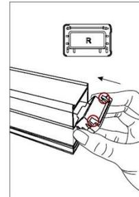
To install Bottom Rail Left and Right End Caps, match the flat side of end caps with the bottom rail of your shade (For bottom rail end caps, left / right side are the same). By using the flat surface on end caps, push fabric/ stiffener against end of rail and slide end caps into side of rail.
