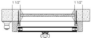
Add 1½" on each side of window opening for max frame-to-frame measurement
