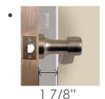
Minimum 1 7/8" from door surface to door handle is needed to leave room for the frame
