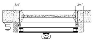
The L-frame design requires a minimum of 3/4" to avoid hitting the glass
