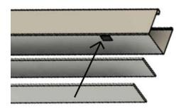
The battery is shipped partially charged. It is a good idea to fully recharge it before installing the blind in the brackets. Connect the USB connector from the Charger to the Battery USB port in the **right hand side** of the head rail as shown.
